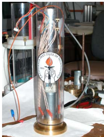
The Caltech cryobot's nose cone. The brass section melts the ice. Photo: Hermann Engelhardt
