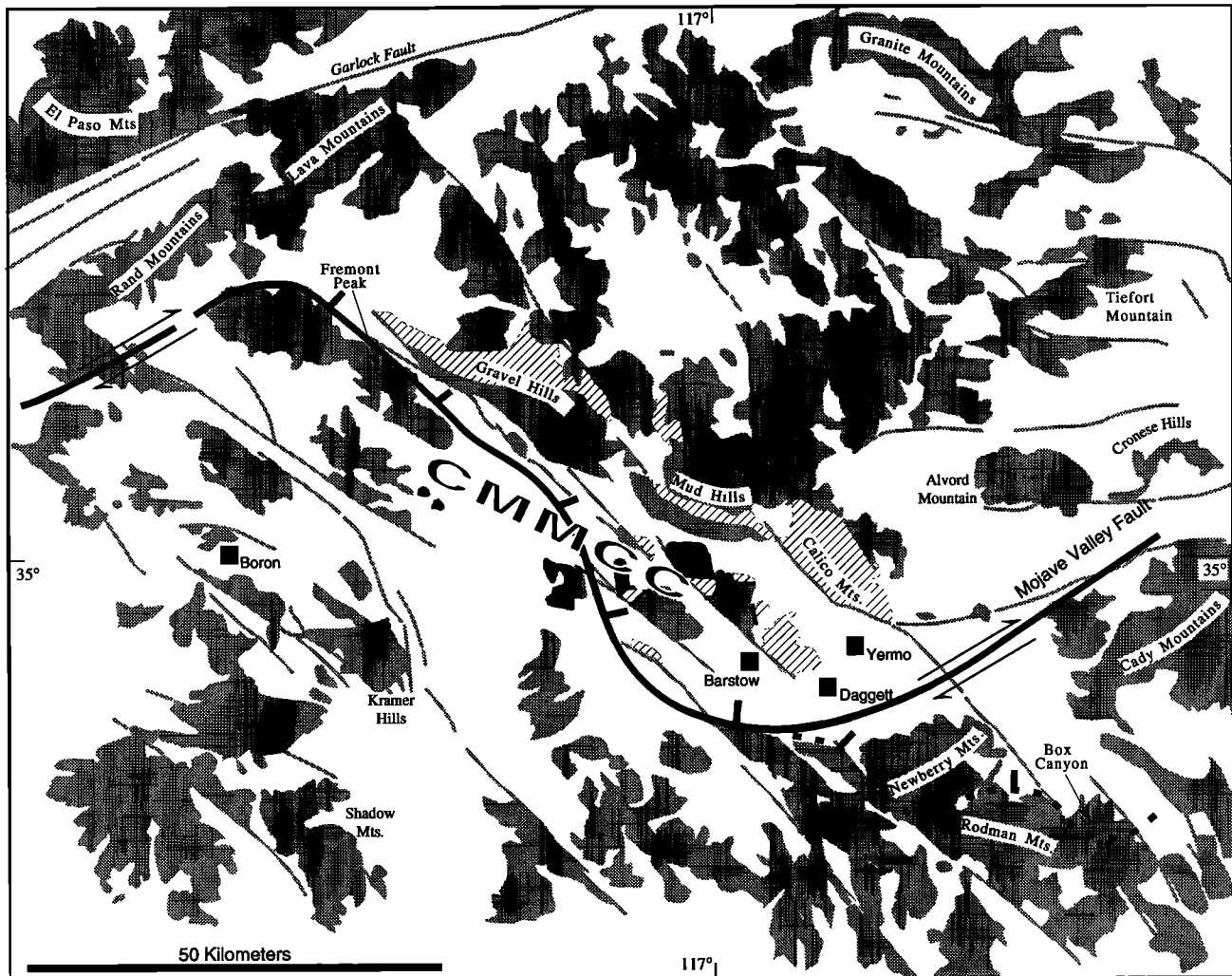
Figure 6. Transfer fault model for the development of the CMMCC. The Waterman Hills detachment fault, the main low-angle normal fault in the CMMCC is shown by bold lines north of Barstow. Miocene sedimentary rocks above the Waterman Hills detachment fault are shown with a diagonal rule. Miocene plutonic rocks in the footwall of the detachment are shown with random dash pattern. The main separation between hanging wall and footwall rocks is shown by bold line with tic marks (on upper plate). Position of the transfer structures are only broadly constrained. Miocene rocks in the Newberry Mountains are age equivalent to the Pickhandle Group: these rocks are south of the Mojave Valley fault (main transfer structure) but are internally somewhat extended. For this reason a splay of the Waterman Hills detachment is drawn into this area.
