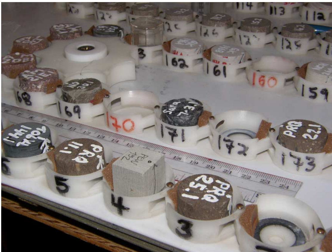
Figure 2. Delrin™ sample-changer cups, arranged in the “snake-chain” assembly. To stop samples from wobbling on a single-point irregularity, a flat rubber “O” ring is glued to the base of each cup. This forces even the most irregular samples to rest on at least 3 widely spaced contact points, which does not always happen with a solid bottom of either plastic or rubber. We also placed a strip of light, self-adhesive weather-stripping foam on the back side of the cups to hold the specimens stable and snugly tangent to the edge of the circular base of each cup while the snake chain is moving. Although this results in the center of a typical specimen being offset by a few millimeters from the center of each cup, the user can tell the instrument what this average offset is for a group of samples via a “fractional hole offset” parameter built into the software. During the sample pickup and drop-off operations, this allows the sample changer to center the specimen itself under the quartz-glass tube while allowing it to pass through the center of one of the bottomless cups for the measurement process.
