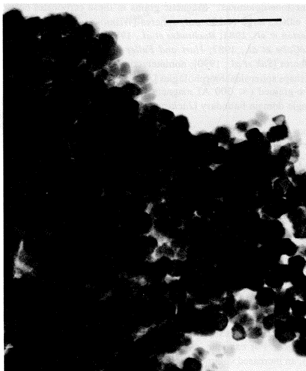
Fig. 2. TEM photomicrograph of single-domain magnetite crystals. The grains often occur as large clusters when separated from the carbonate matrix of loose sediment, limestones, and dolomites. The effect of the separation technique on clustering is uncertain. Sample from Ocean Drilling Program Leg 101, site 632-5H, 125-129 cm. Scale bar 0.5 \mu\text{m} .
